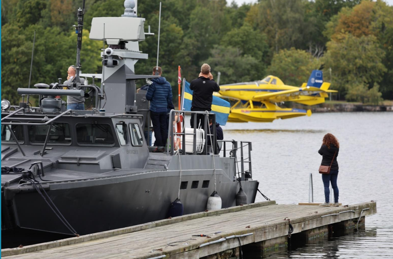
Figure 21. The Autonomous Combat Boat 90 "Enforcer III" from Saab Kockums equipped with Camera sensors from Axis Communications serves as a floating lab both for WARA-PS and other projects. A manually operated Saab Fireboss (Air Tractor AT-802) picks up water to drop at requested spot.
