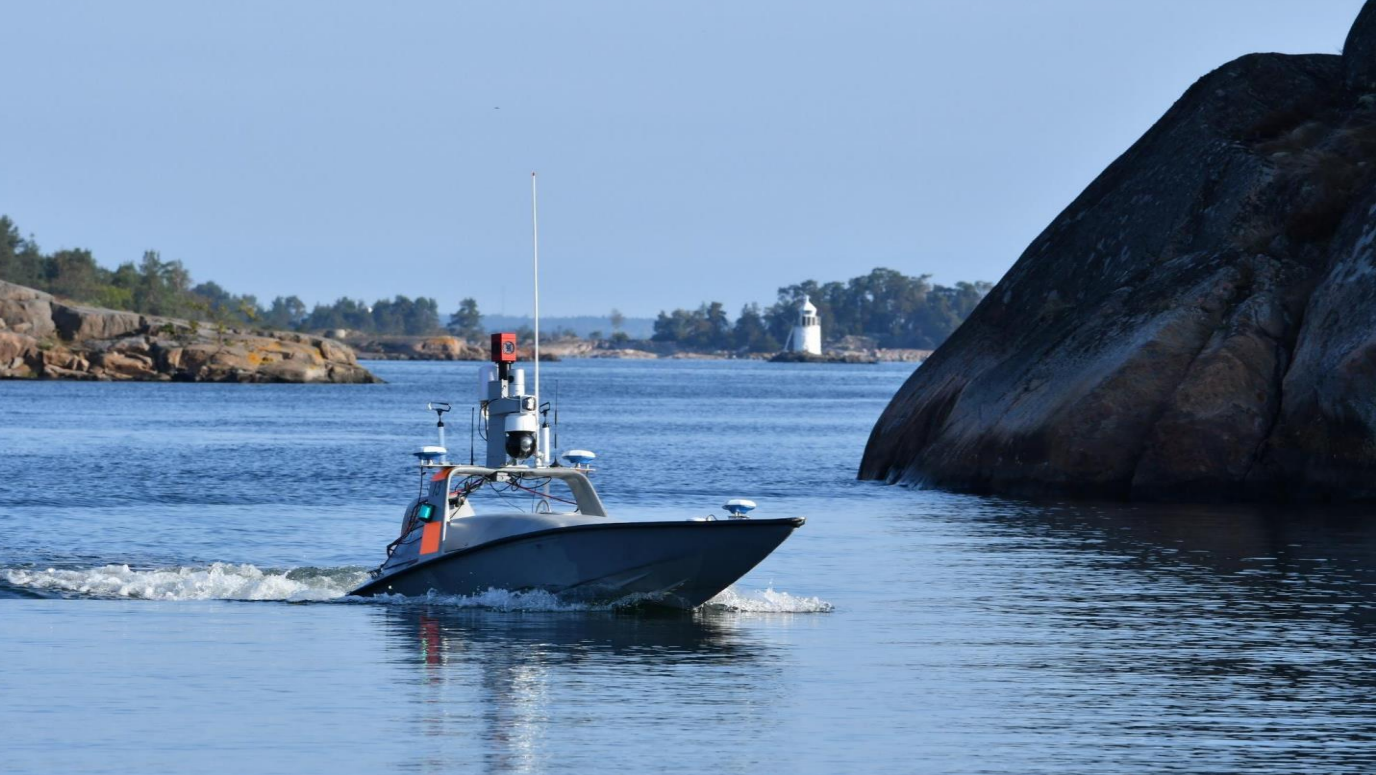
Figure 6. GPS Free Positioning – Neural networks, Bertil Grelsson, LiU 2018-2019. The Piraya from Saab Kockums on a data collection run in the archipelago outside Gränsö/Västervik 2018. On top of the boat is a 360-degree camera mounted, recording the surrounding terrain together with reference positions. The dataset created was used in Bertil Grelssons PhD thesis.
