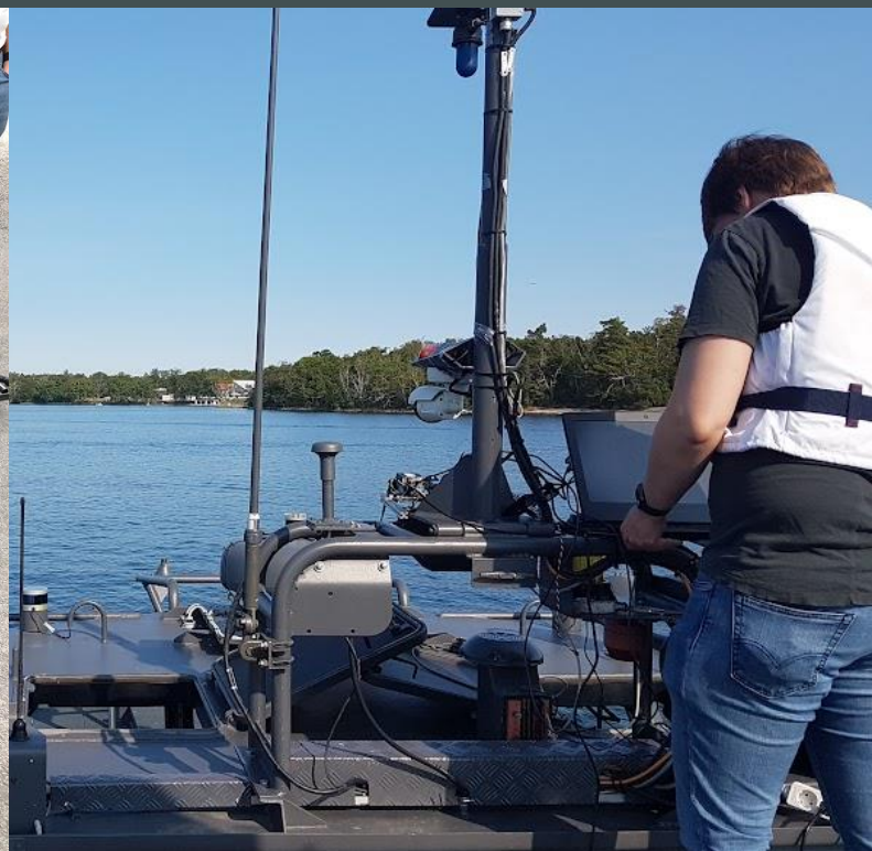
Figure 22. There are also spontaneous resources showing up at events. The photo show Gustav Häger, LiU, working with stereo cameras and LIDAR on (right) Combat Boat 90 "Enforcer III" and the same system on (right) a Gränsö hotel On-site-built "Drink wagon" as a hardware emulation of the moving boat. More stable than the offered Golf car. A good example of cooperation between PhD students, hotel manager Per Johansson and Lars Rundqwis.
