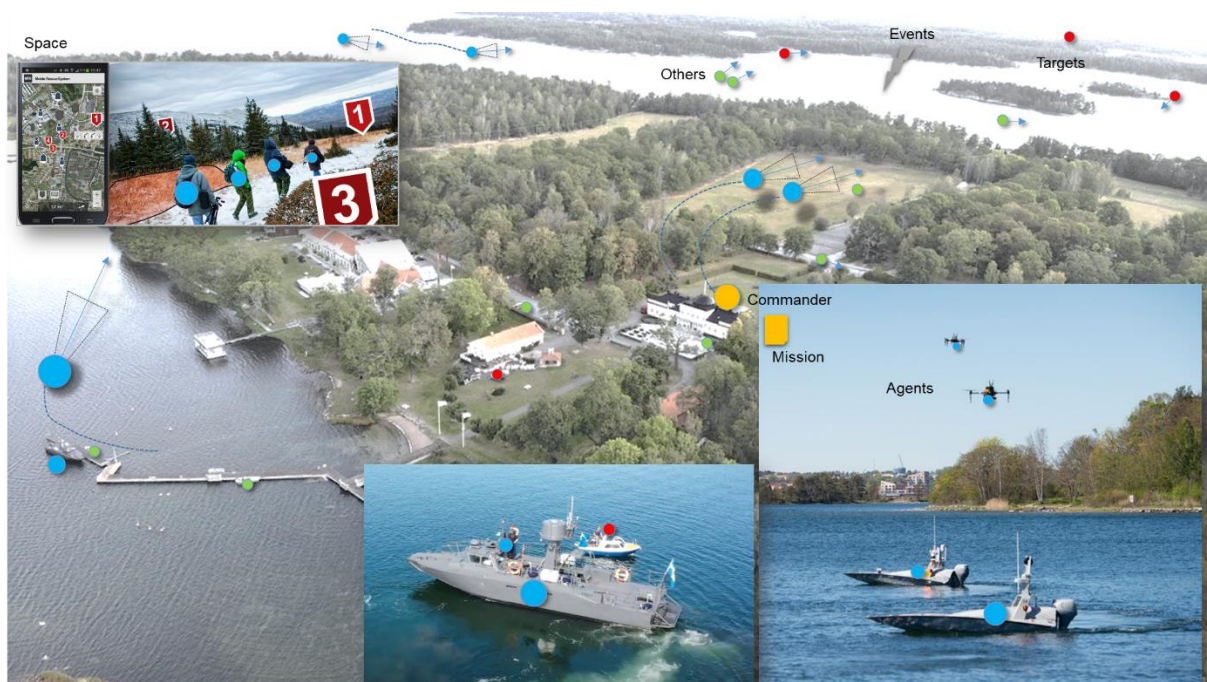
Figure 23. A Search and rescue scenario overview where the Gränsö environment are used together with Core system and resources. This figure shows an example mission where blue search agents trying to find missing red agents and distinguish them from the green not interesting agents. A grey agent act as a commander directing and follows up the mission. Agents are a mix of human and robots.
